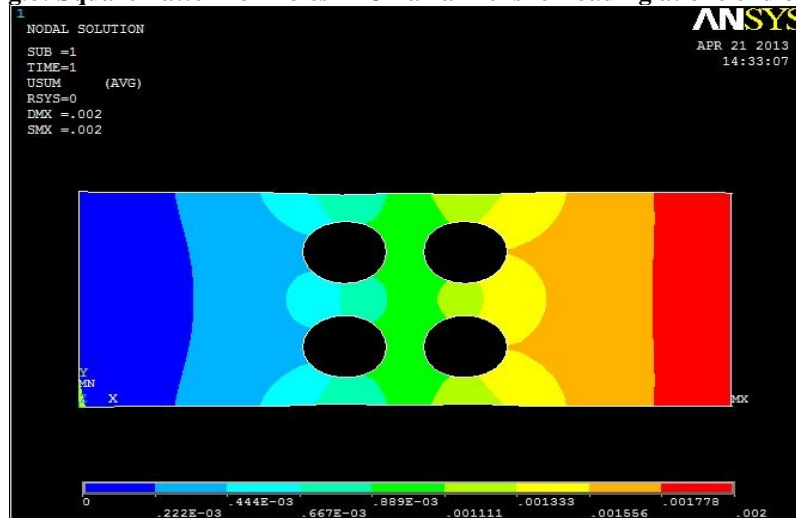
Fig.9: Deflection for Plate with Square Pattern of Holes
